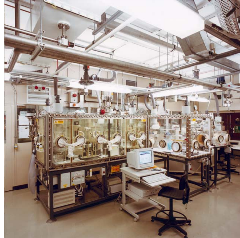
OSL Sellafield. (Since 1999) Robotic system for small spiking, separation chemistry and alpha counting
