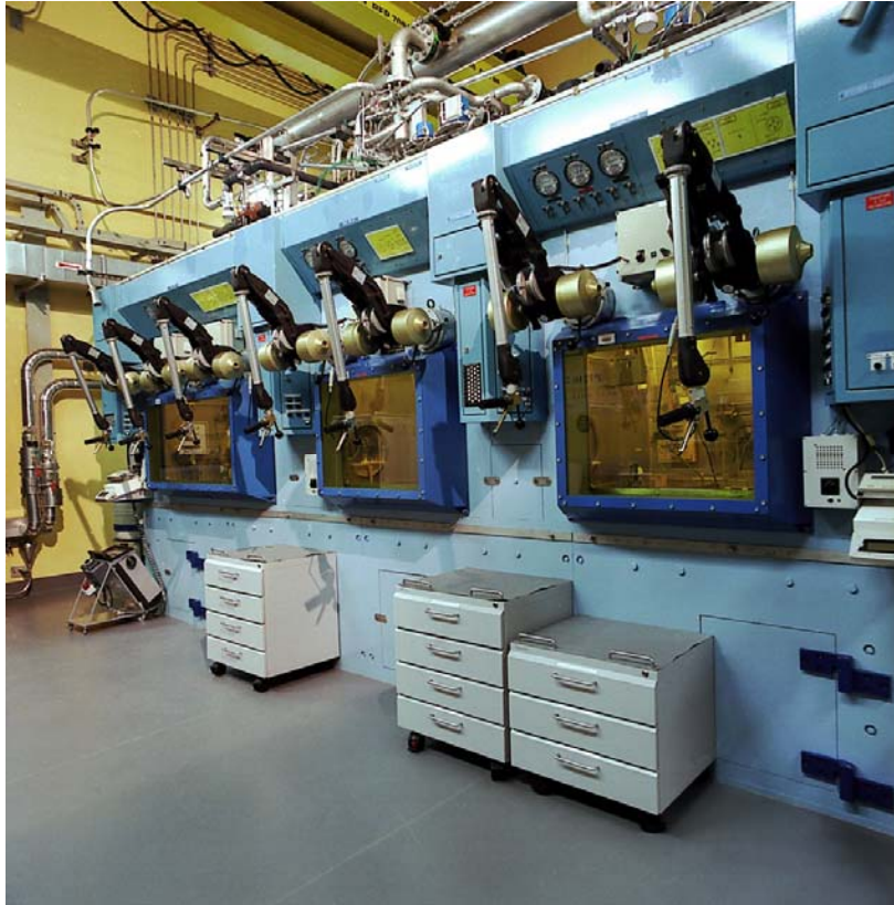
LSS La Hague. (Since 2000) Hotcells for handling dissolved spent fuel samples.
